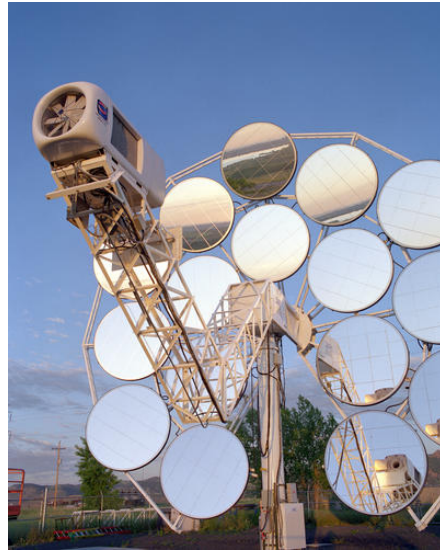
Photo 7 – Solar Parabolic Dish Sterling Test System
