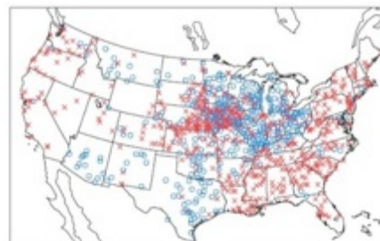
Figure 1. Location of stations with less than 10% missing daily precipitation data for 1895–2000. The symbol 'o' (in blue) indicates that long-term data were available prior to CDMP while the symbol 'x' (in red) indicates newly available long-term stations.
