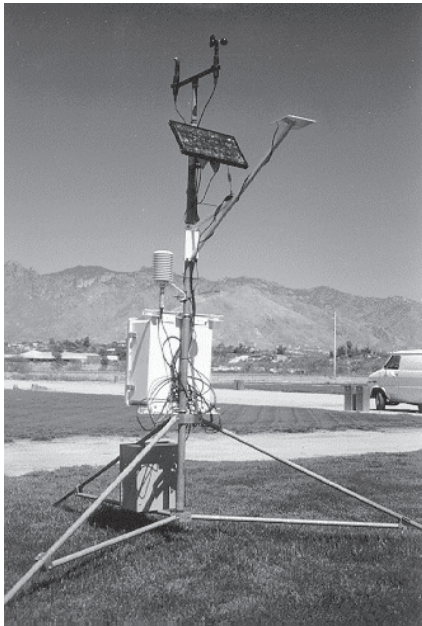
Figure 2. A 10-foot tower supports instruments that measure air and soil temperatures, humidity, solar radiation, wind speed, wind direction, and precipitation at an AZMET station in Tucson.
